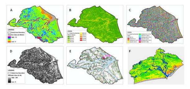
Figure - 4: Topographical Maps, A - ASTER - DEM with 30 m Spatial Resolution, B - Slope Map, C - Aspect Map, D - Hillshade Map, E - Toposheet (1:25,000 Scale), and F - 3D View of the Study Area
