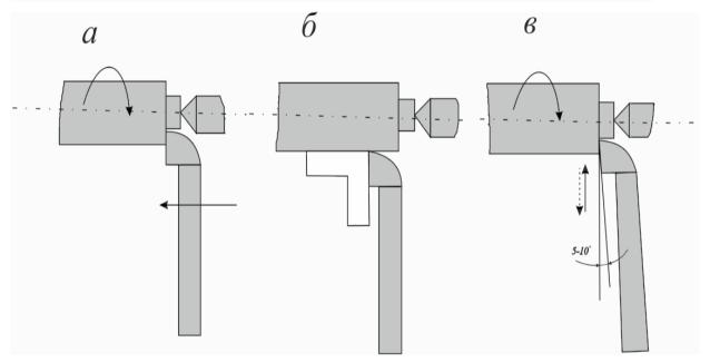
In order to use cutters with an angle of 90° between the steps of the stepped shaft. The pinole in the housing is installed at an angle of 15°, and the transition ledges on the copier have an inclination to the axis of 75°. Therefore, the cutter moves away from the part in a direction perpendicular to its axis.
