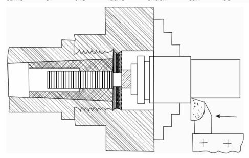
When choosing and operating through-hole cutters, their different durability should also be taken into account (the time of direct work from sharpening to overfilling). Under equal conditions, thrust incisors are less resistant, having a sharper and less durable tip, prone to overheating.
