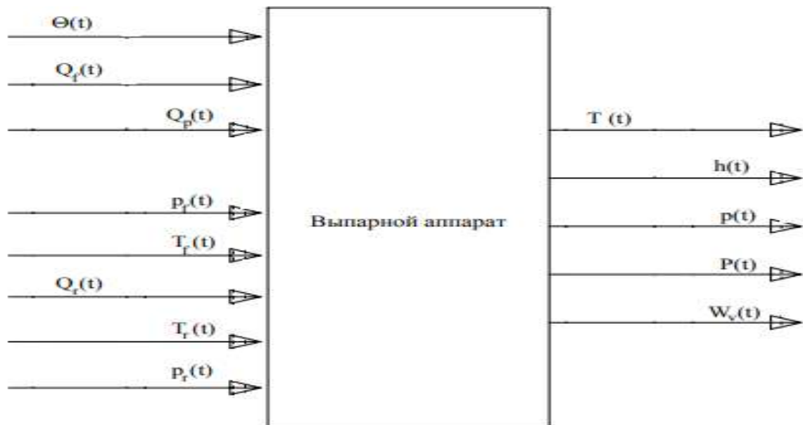
Fig.2. Composition of the main variables of the computer model of the evaporation apparatus
