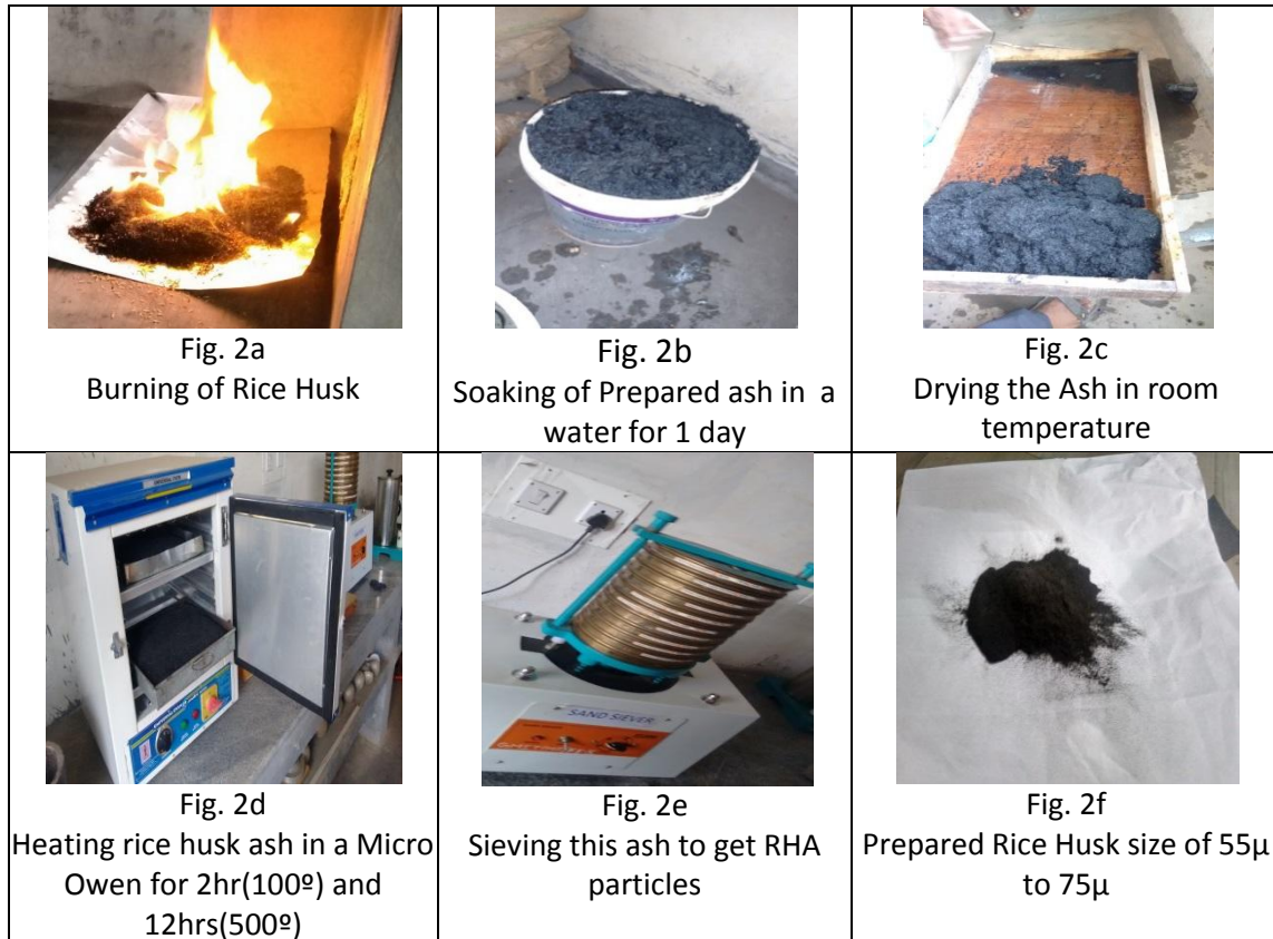
Fig. 2: Step wise Preparation of RHA
