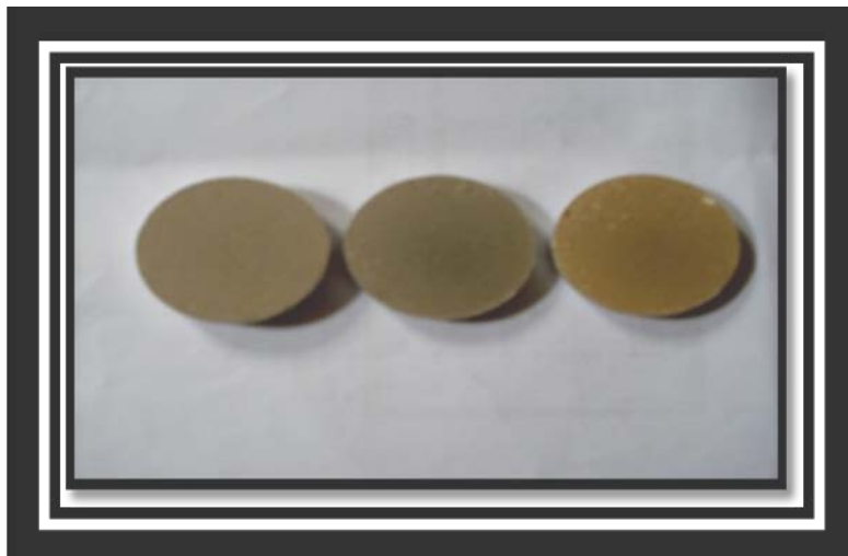
Figure 2 showing some solidified samples (Pallets) ready for XRF analysis. (Photograph by the author at SAIF, G.U.).
