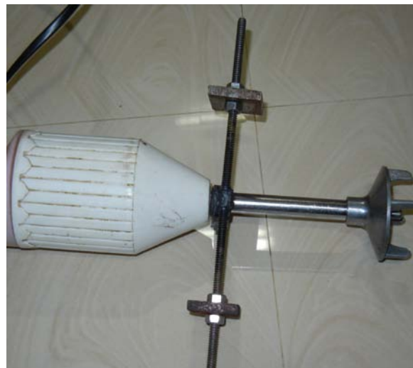
Figure 6: Hand blender with TVA
