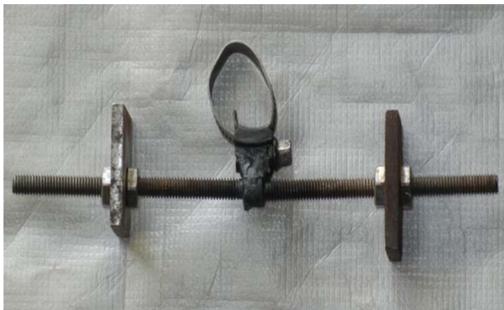
Figure 3: Dual mass TVA
