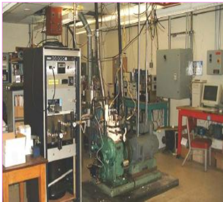
Figure: 5 Research engine with variable valve actuation system
