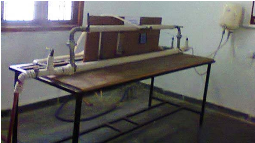
Fig.2 practically developed model of heat exchanger for parallel and counter flow
