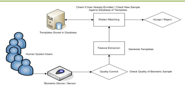
The working procedure of any biometric system includes the following three phases.
