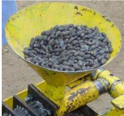
Figure 6 Simple ram press used for oil extraction
