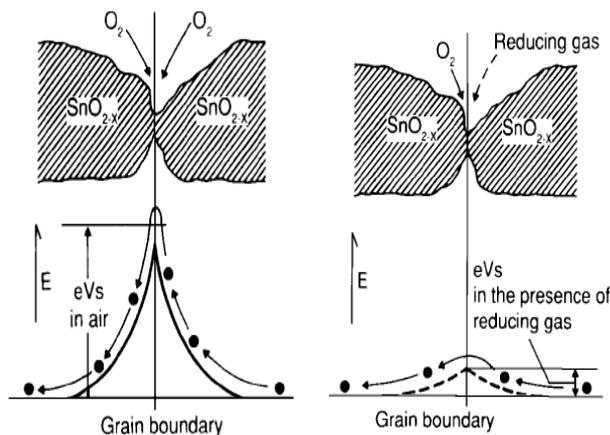
**Figure 1. (b) Gas sensor working principle**
