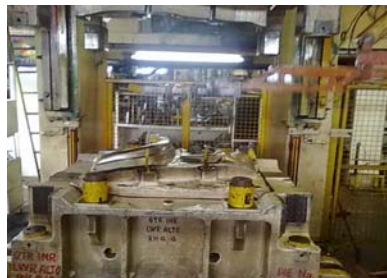
Fig.4: The re-striking operation of rear lower housing.
