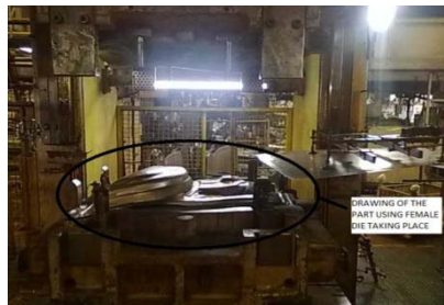
Fig.1: The drawing operation of rear lower housing.
