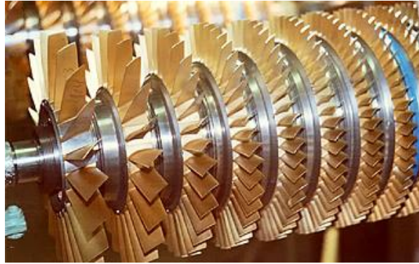
Picture 1 - Compressor Assembly
