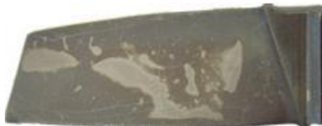
Picture 1 - Eroded Compressor Blade
