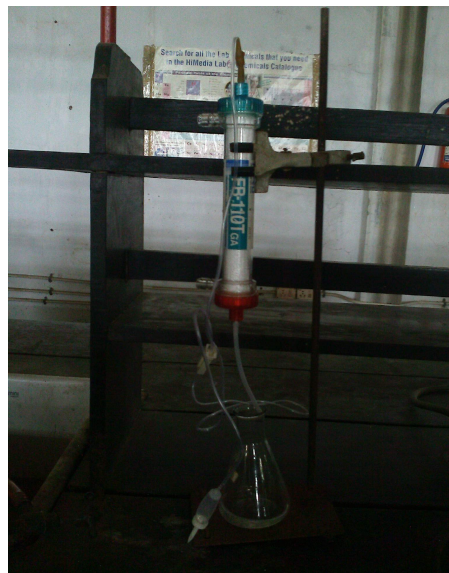
Figure 3: The reverse osmosis column
