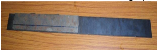
Figure 9(e) Steel Beam with 50% coverage of CLD with steel constraining layer
