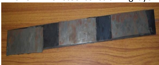
Figure 9(i) Steel Beam with multiple of CLD with steel constraining layer (each patch is of 150 mm length)
