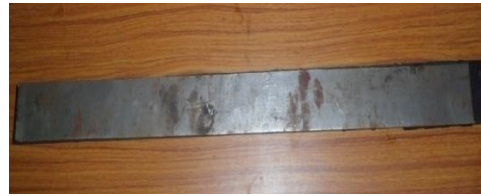
Figure 9(b) Steel Beam with full coverage of CLD with steel constraining layer
