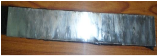
Fig 9(a) steel Beam with full coverage of CLD with Aluminum constraining layer
