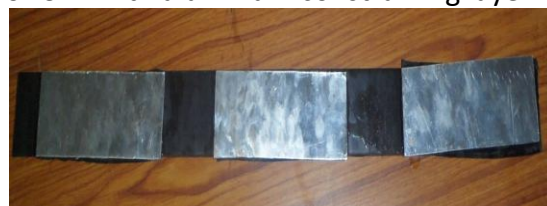
Figure 9(j) Steel Beam with multiple of CLD with aluminum constraining layer (each patch is of 150 mm length)
