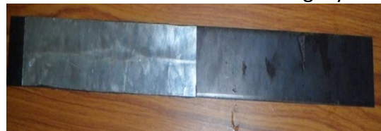
Figure 9(f) Steel Beam with 50% coverage of CLD with aluminum constraining layer
