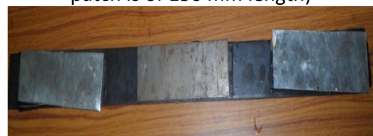
Figure 9(k) Steel Beam with hybrid CLD (middle steel layer and edge aluminum layer)
