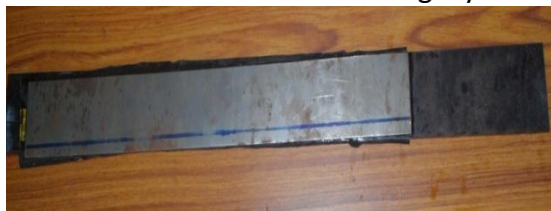
Figure 9(g) Steel Beam with 75% coverage of CLD with steel constraining layer
