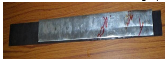
Figure 9(h) Steel Beam with 75% coverage of CLD with aluminum constraining layer
