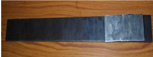
Figure 9(c) Steel Beam with 25% coverage of CLD with aluminum constraining layer
