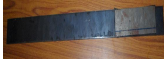
Figure 9(d) Steel Beam with 25% coverage of CLD with steel constraining layer
