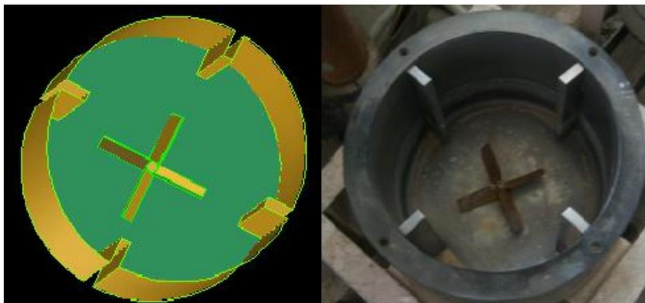
**Figure 3: a) CAD model of fluid volume with propeller b) Cylinder with propeller**
