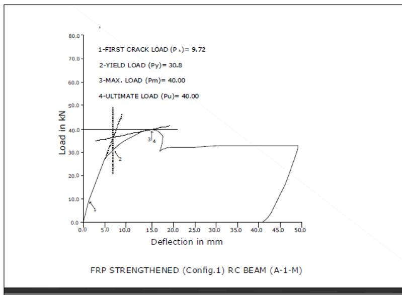
FIG.6: Load- Deflection Curve under Monotonic Loading Test (Beam Specimen A-1-M)
