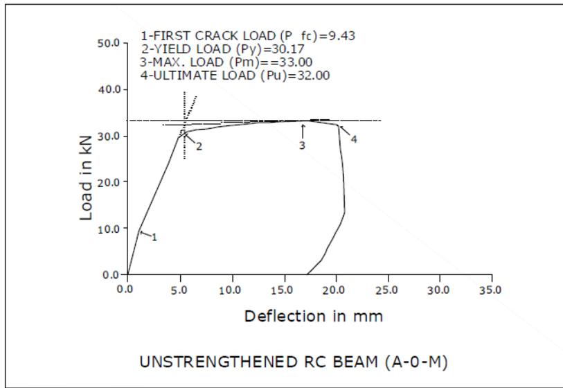
FIG. 5: Load- Deflection Curve under Monotonic Loading Test (Beam Specimen A-0-M)
