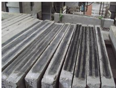
FIG. 2 : FRP APPLIED BEAMS LEFT FOR AIR CURING
